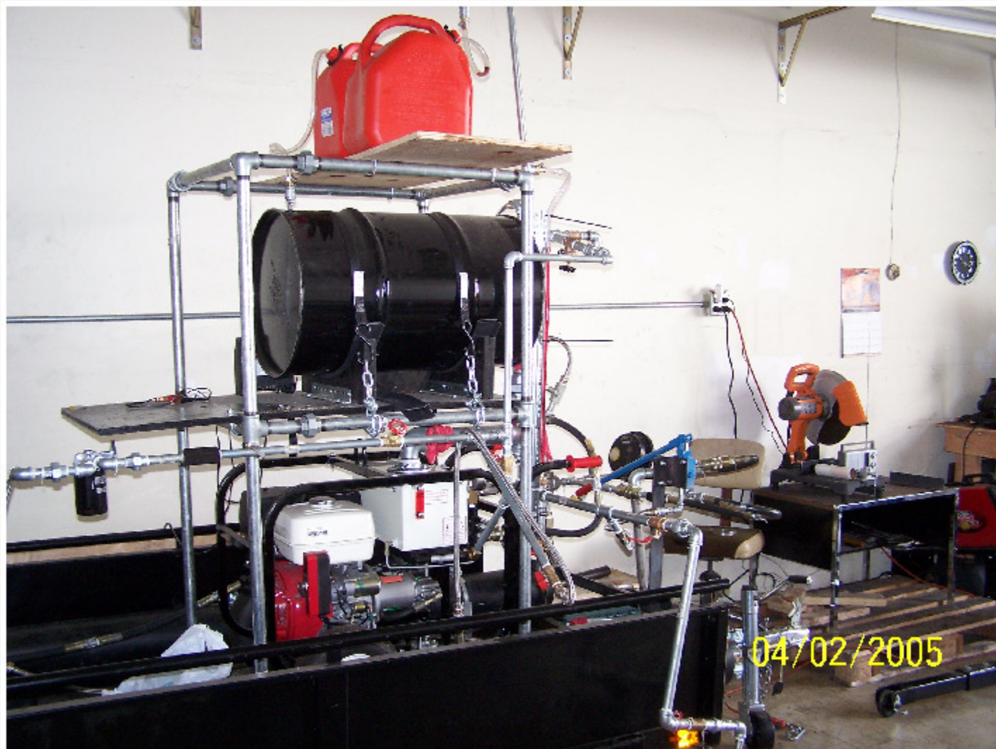
10 HORSE POWER 3000 PSI HYDRAULIC POWER UNIT, 30 GALLON RESERVOR TANK AIR / OIL ACCUMULATORS ALL MOUNTED ON 4 FT X 8 FT TRAILER
