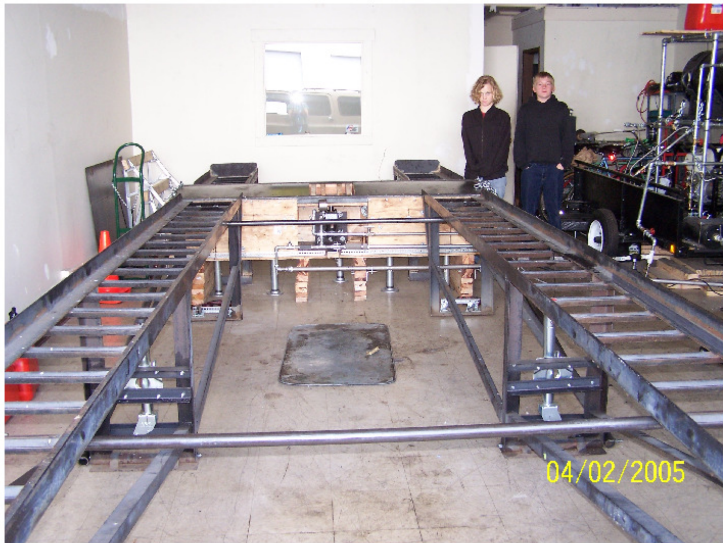
SPEEDBUMP ATTACHED TO VEHICULAR DISPLAY RAMPS FOR TESTING PROTOTYPE
