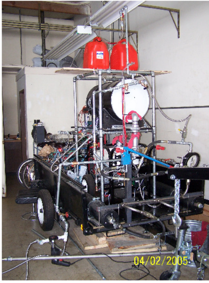
10 HORSE POWER 3000 PSI HYDRAULIC POWER UNIT, 30 GALLON RESERVOIR TANK AIR / OIL ACCUMULATORS ALL MOUNTED ON 4 FT X 8 FT TRAILER
